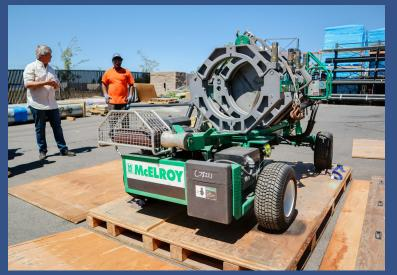
The Rolling 618 bridges the gap between small and large diameter fusion, and incorporates a universal 4-jaw carriage that can be easily removed for fusion operations remote from the vehicle. For installations in limited space, the outer fixed jaw and skid can be removed from the carriage, converting to a 3-jaw carriage for close access in tight installations.
